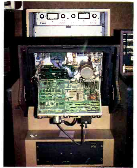
View of the front of the machine with the tape transport raised. The electronics shown on the bottom are the analog and digital logic circuits, which control all the tape transport functions.
