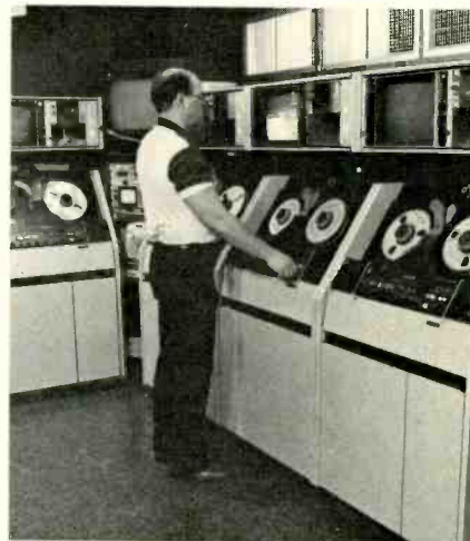
Video West's central tape operations room contains six Ampex VPR-2B 1-inch VTRs.
