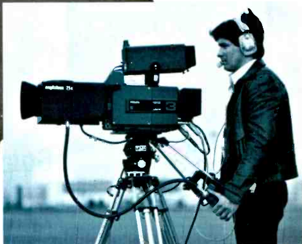
LDK14S in studio and field mode. Digital techniques in the camera and base station (RCU) require only an adapter for triax conversion... another LDK14S cost advantage from the originator of triax... Philips.
