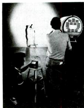
Photocell centered in beam with remote meter scale near lamphead.
