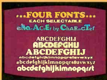
MULTIFONT DISPLAY Up to four fonts from the font library can be loaded from the disc and mixed on a character by character basis.
