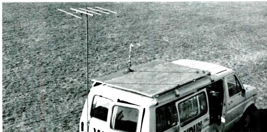
The van, equipped with a directional antenna, is prepared for a remote transmission.
