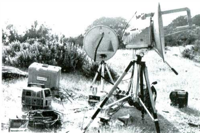
KRON-TV use the 700-foot peak at Valley View Hill just below the Diablo Canyon plant at Port San Luis as the first in a series of eight microwave hops to the station in San Francisco.
