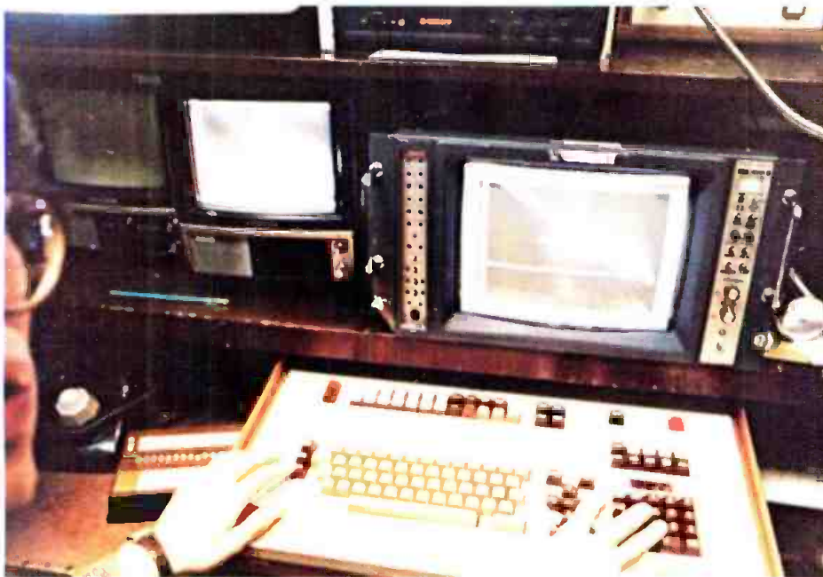
One line of the 525 lines of the video image can be isolated for graphic alteration.
