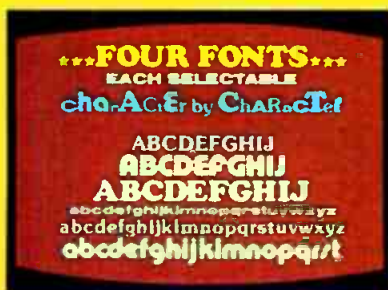
MULTIFONT DISPLAY Up to four fonts from the font library can be loaded from the disc and mixed on a character basis.
