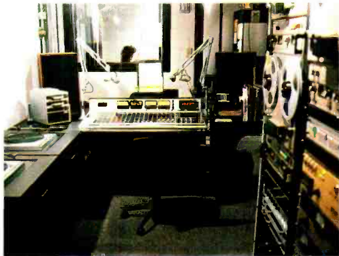
From the back of the main control room, we see the spatial relationship between the equipment racks and the on-air operating position. Turntables, carts and remote controls for the tape decks are close at hand for maximum operating convenience.
