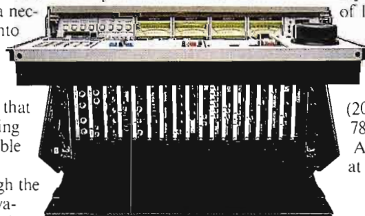
Front access to all electronic circuits and modules.
