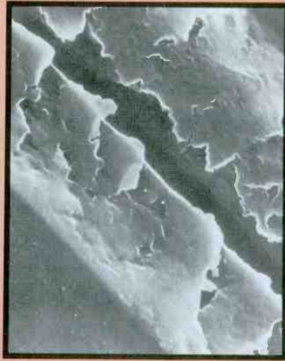
A 45 rpm disc shows peeling of the outer shell of polystyrene material after backcueing 10 times with a spherical tip. (magnified 10,000X)
