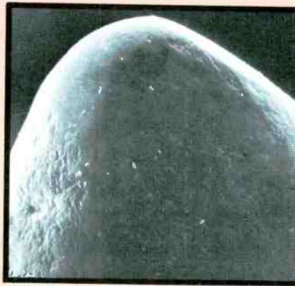
An elliptical stylus beginning to wear at approximately 100 hours of use. (magnified 3000X)
