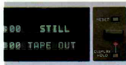
Display board for self-diagnostics and other data-processing functions.
