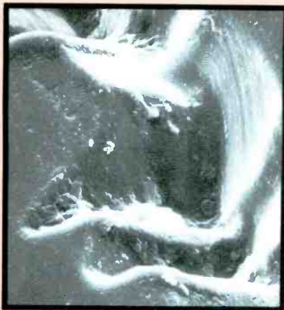
A disc with high groove modulation, as found in many modern recordings. Such modulation would be almost impossible to trace properly. (magnified 2000X)
