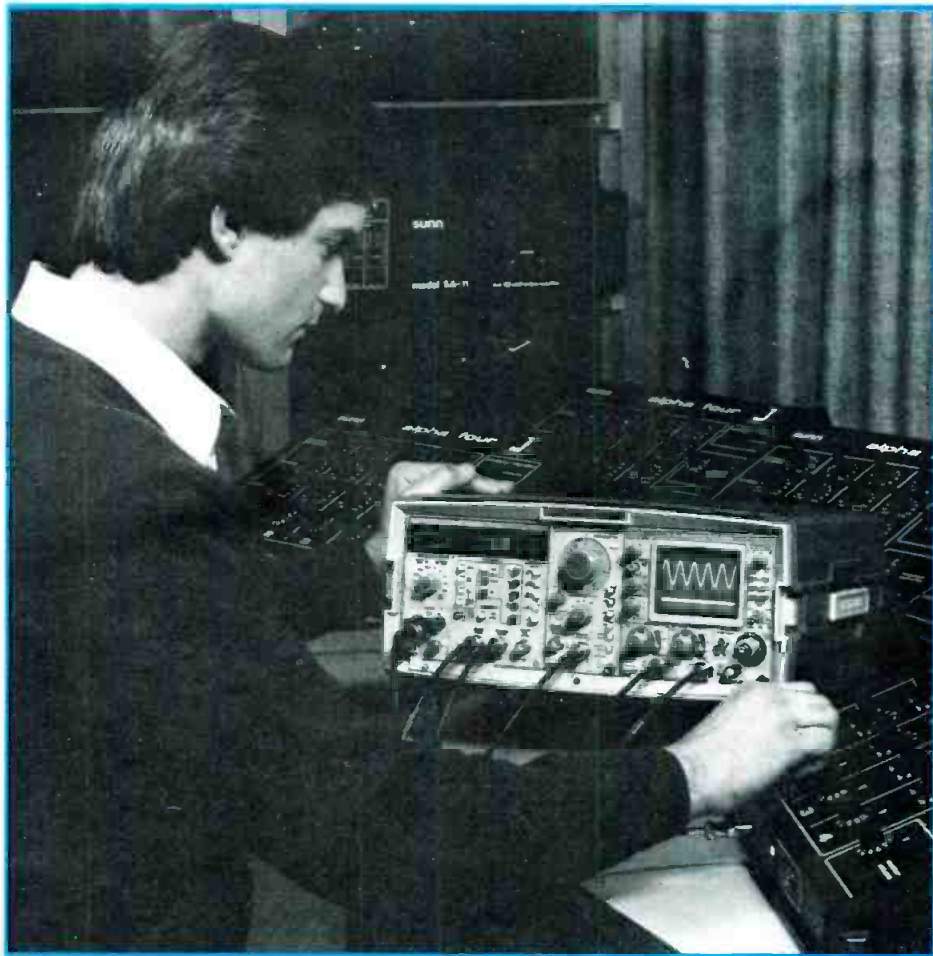
A technician uses the AA 501/SG 505 system to check performance of a small audio mixing system. For his tests, the system includes an SC 503 10MHz storage oscilloscope.
