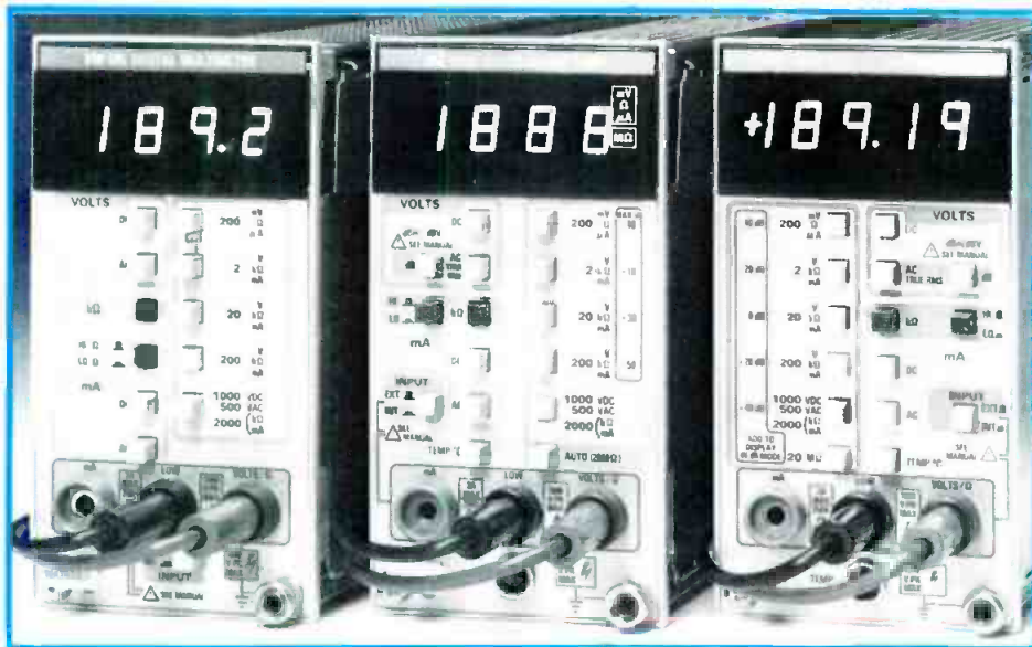
Any one of the DM 502A, DM 501A and DM 505 autoranging DMMs may be selected for use with the distortion analyzer/signal generator set.
