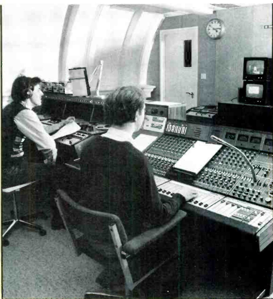
The 24-channel mixing equipment in the new sound studio.
