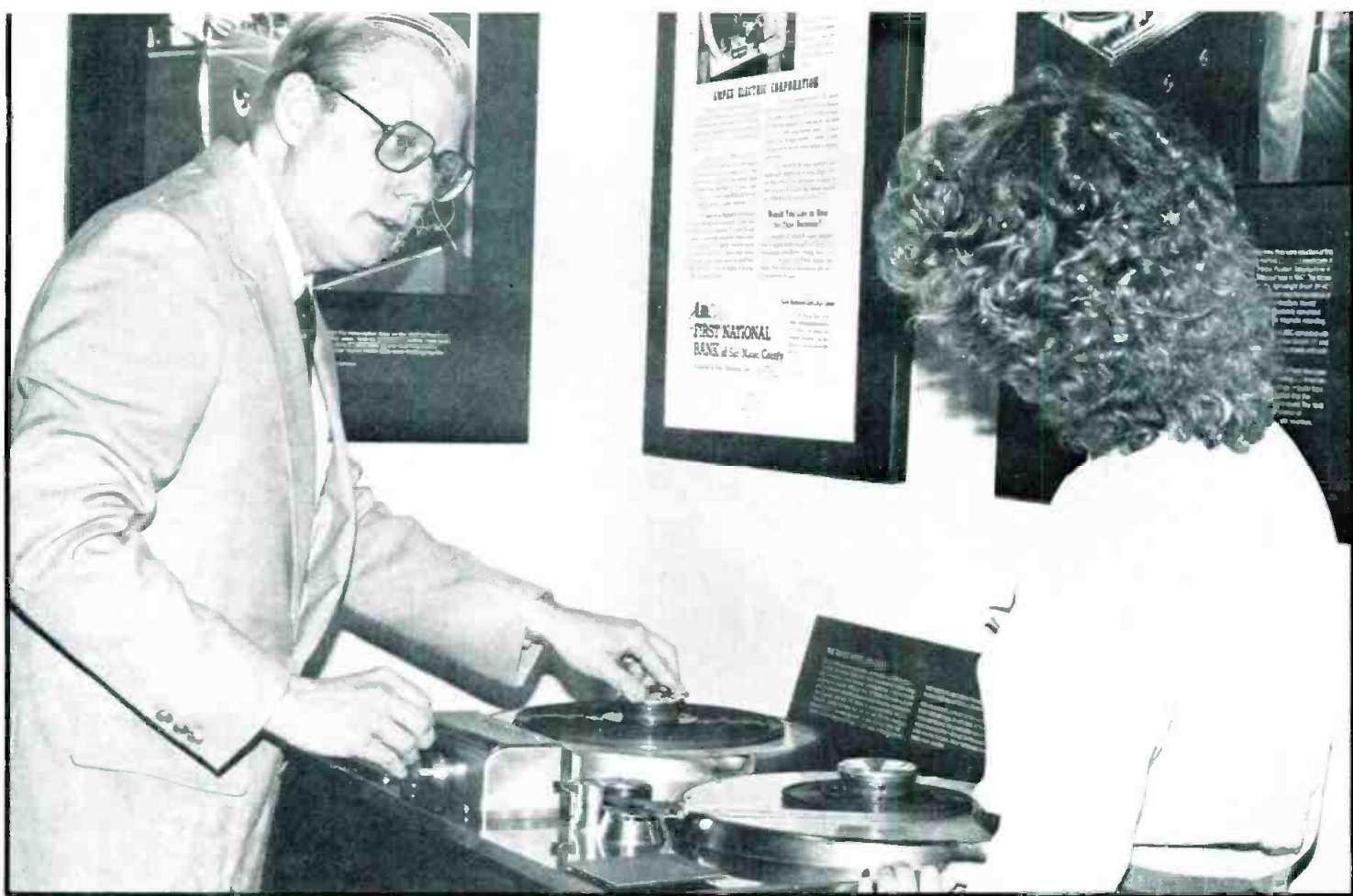
Hammer reviews the features of an Ampex model 200, the first successful tape recorder produced in the United States. The machine, introduced in 1948, produced just one channel of audio.
