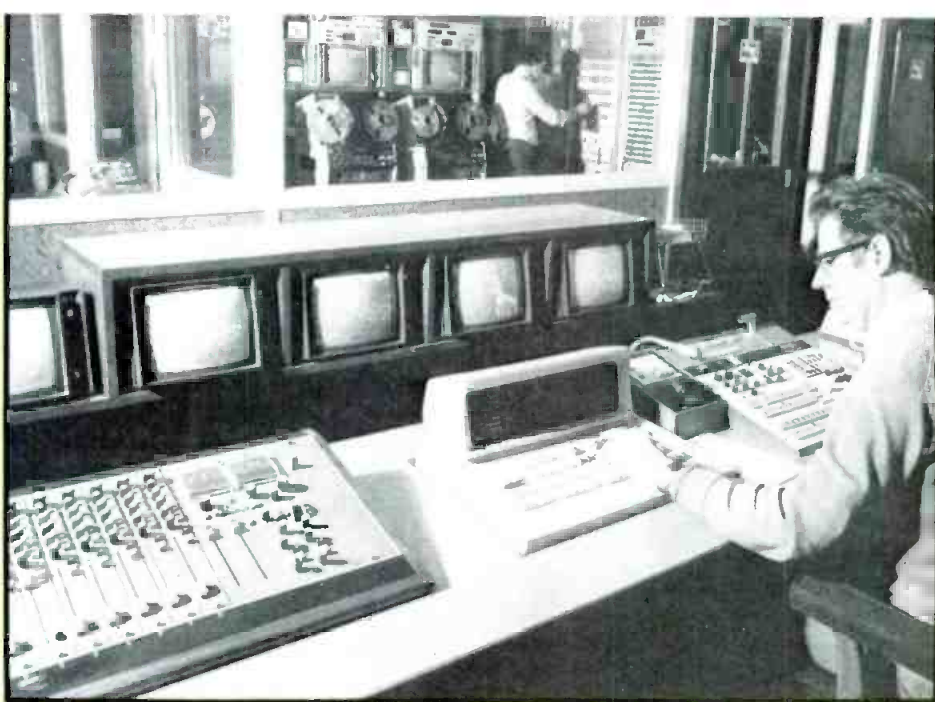
The editing control computer operating the VPR2 machines in the new editing suite, showing the sound and picture control consoles.
