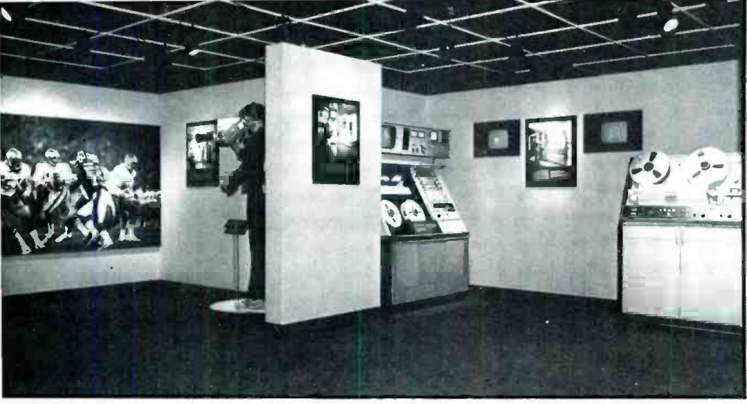
Also included is a display of videotape recorders produced since 1956. The mannequin at the left is holding an Ampex VR-3000, the first portable VTR, introduced in 1967. The larger recorder in the center is an Ampex AVR-1, the industry's first modular system, and to the right is an Ampex VR-2000, the first high band color VTR, introduced in 1964. Not shown is an RCA TR22 VTR, the first all-transistor system.
