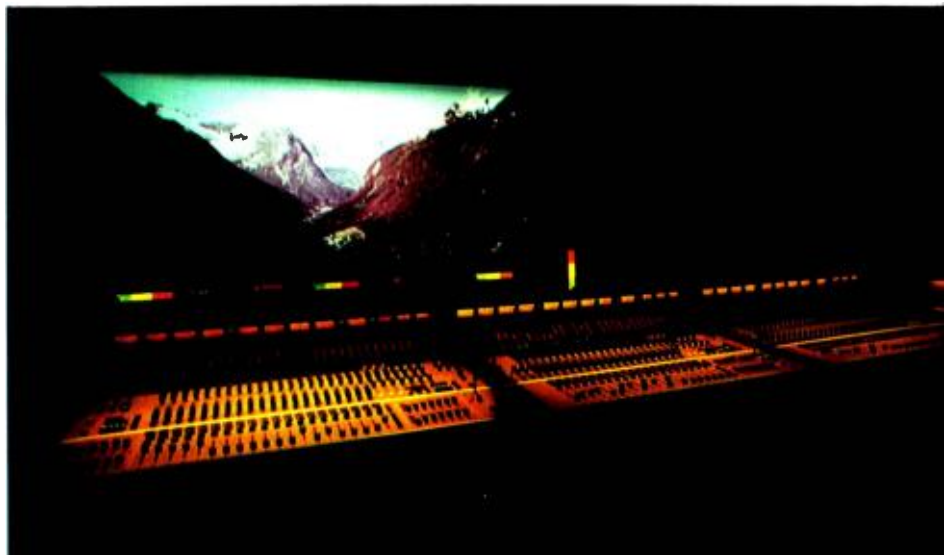
An ADM custom stereo system for Glen Glenn, Hollywood, includes 96 inputs and 18 outputs with microprocessor control and interfacing into the total post-production system.
