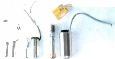
Shown (from right) are 25mm, 17mm and 13mm pickup tubes and yoke assemblies.
