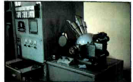
Flying spot scanner constructed in China.
