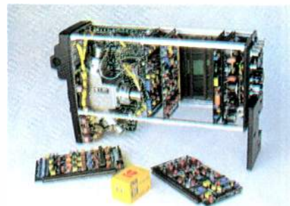
TC-90 camera, with housing removed, shows internal construction.
