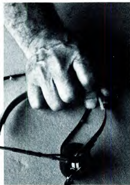
Shown is a CBS field invention, an announcer's headphone/mic, which uses a Sony headphone, a Plantronics boom and a tiny Tram mic with windscreen.
