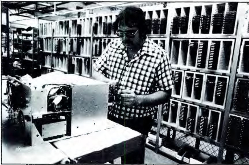
Boards are married to wired chassis in the subassembly area.
