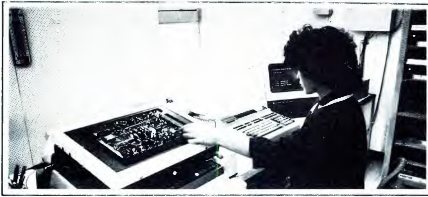
A Hewlett-Packard automatic test system provides total testing of printed circuit boards.
