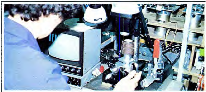
Special instrumentation is required to check the speeds of an MTR-90 capstan-drive unit. An electron microscope produces a video display to help locate the capstan encoder.
