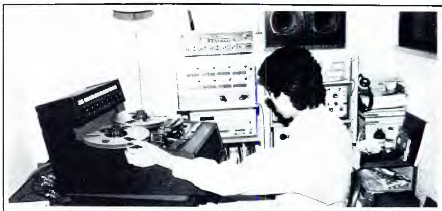
Once completely assembled and checked, an MX-5050B Mark III-8 is again tested before crating for shipment.
