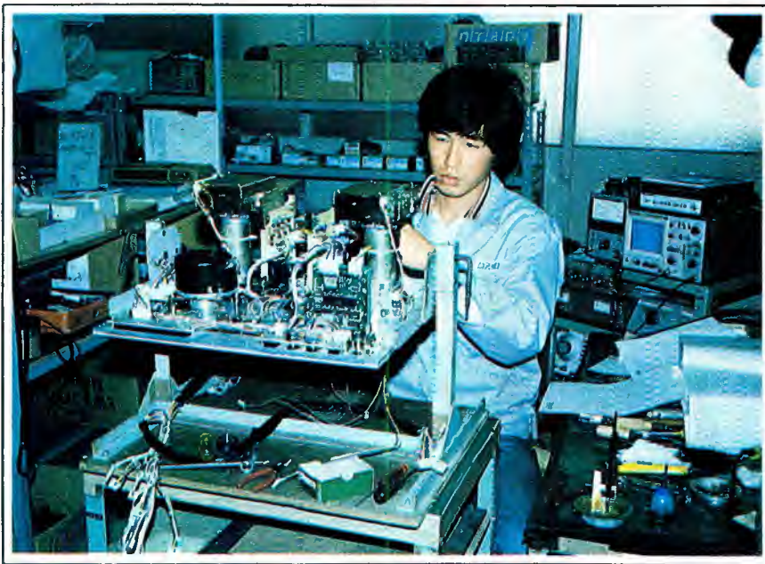
Adjustments are made to the MTR-10 mainframe.
