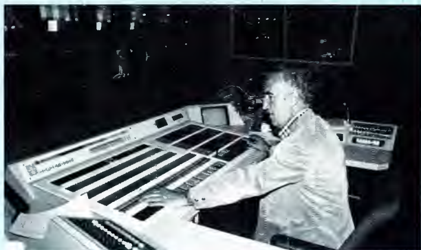
Gil Miller, technical director, operates the new Ampex video switcher in CBS Control Room 41.
