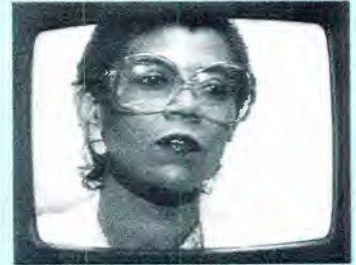
Out-of-band carrier interference eliminated with a bandpass filter.
