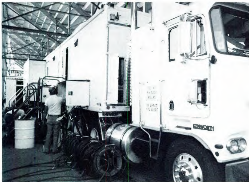
This CBS production trailer's unique construction allows side to expand, enlarging program control room.
