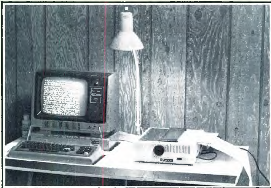
The Radio Shack model 1 computer and less expensive printer are shown. Disc drives for the system are on a lower shelf of the table.
