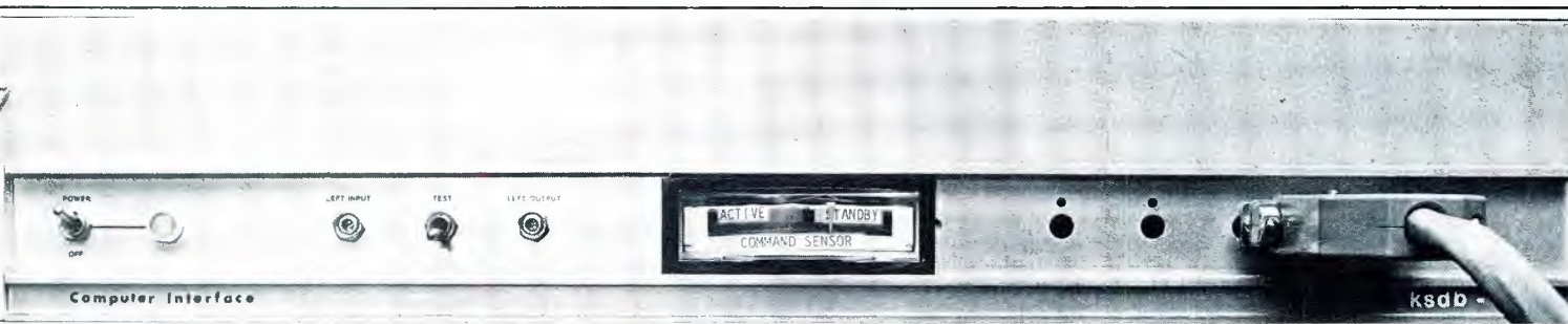
The power supply, unique logic circuitry and relays of the Automate-64 system fit in a 2-inch-high standard rack.
