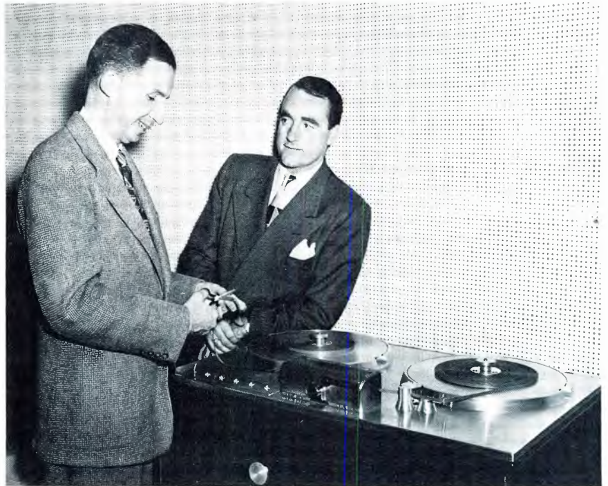
In this 1947 photo, Jack Mullin (left) shows Murdo MacKenzie, Bing Crosby's technical producer, how to edit tape using a pair of scissors. Shown is the Ampex model 200 prototype. In 1945, Mullin had sent two German AEG Magnetophons and 50 reels of BASF/Agfa tape home to San Francisco, where he modified them with ac bias and other improvements. Mullin's Magnetophons later inspired that first Ampex machine.
