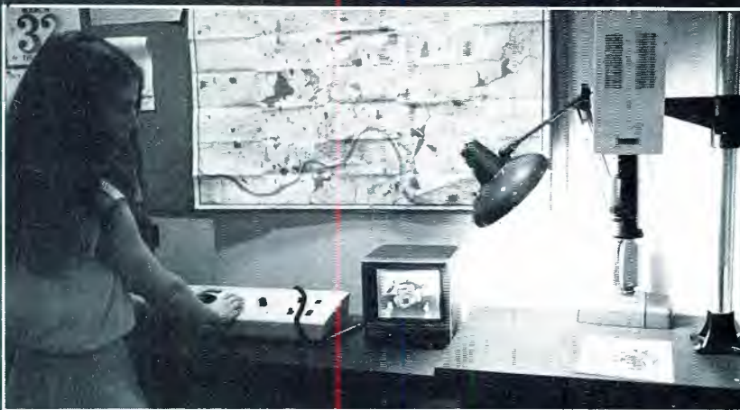
Goodall uses a simple, monochrome camera to digitize graphics from the copystand, then to add color.
