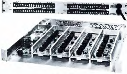
1 R.U. Distribution Frame
