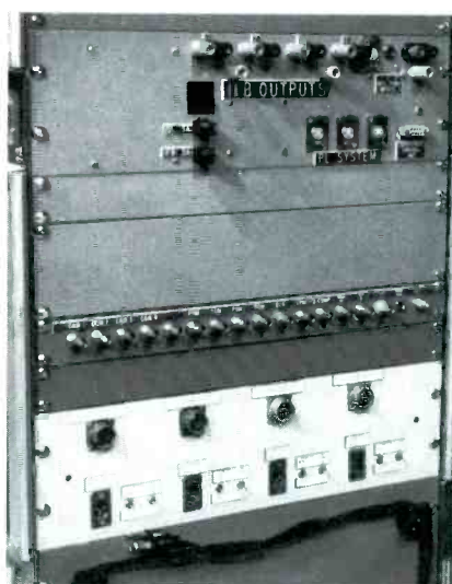
IFB/PL circuitry, video patching and camera inputs easily fit into a single case.
