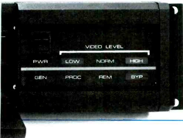
The 550's "put it anywhere" remote panel. Two will fit side-by-side in a 1 3/4" rack space.
