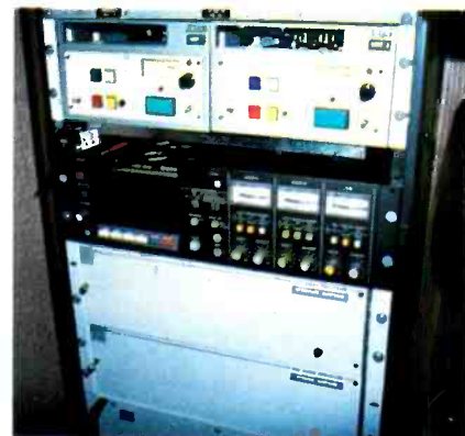
In addition to cartridge audio, a TASCAM 133 cassette recorder/player is available in the audio area.
