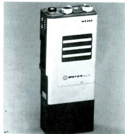
Motorola Electronics MX300 series Handie-Talkie FM 2-way radio featuring frequency-synthesized operation.
