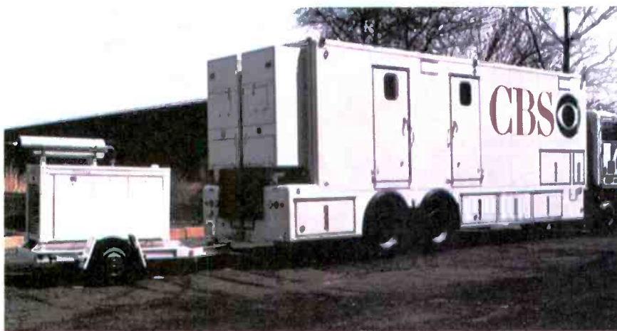
Viewed from the back, Mobile Unit #10 carries its own air conditioners and may tow a power generator, if required.
