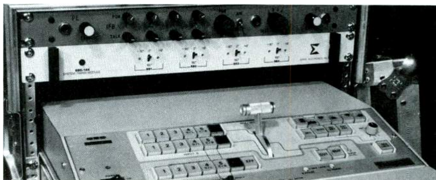
The Panasonic WJ-4600B is slide-mounted in one of the transport cases, with easy access to Sigma Electronics phasing equipment and the communications system level controls.
