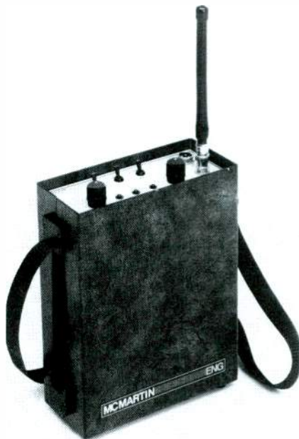
McMartin Industries RPU-1103 3W portable transmitter with a rubber duck antenna attached.
