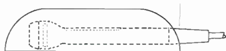
Figure 8. The Electro-Voice 411 Mike Mouse barrier adapter, which is used to hold a mic in the near-barrier position for minimum phase cancellation.
