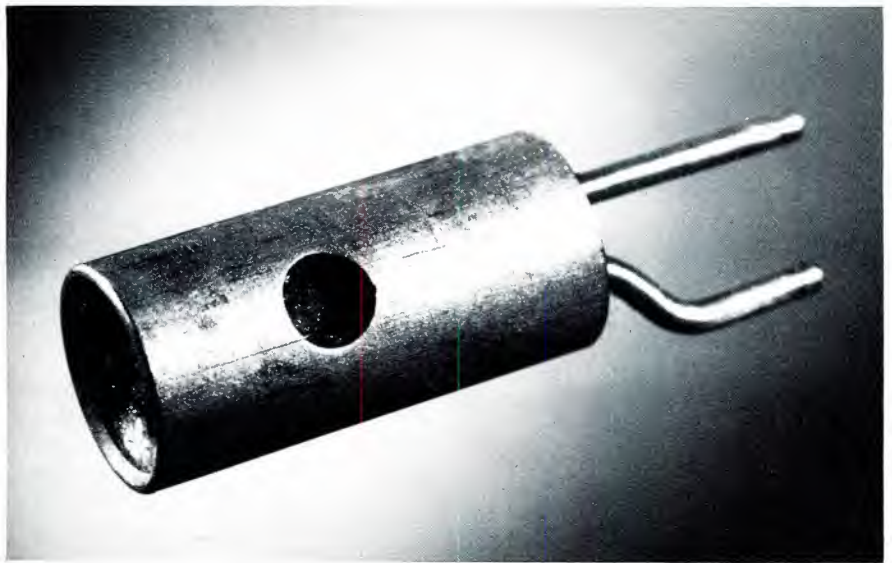
Shown is the first point-contact transistor (Bell Labs code number 1A) to find commercial use in the United States. Although announced to the public in 1948, it was 1952 before transistors similar to this one assumed an active role in the Bell System communications network.
