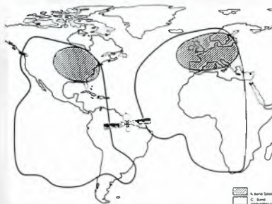
Figure 1. INTELSAT IBS C-Band coverage from 53° west longitude is shown by the shaded circled areas on the map. Ku-Band spot beams, indicated by the striped areas, are steerable over a wide range that could include the West Coast of North America.
