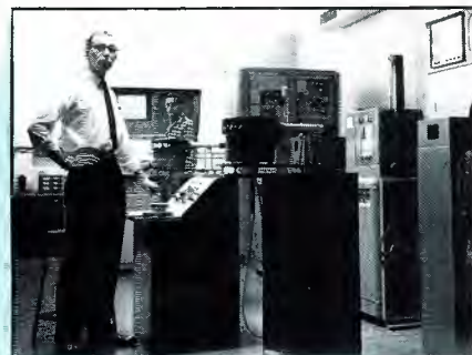
Shown is a portion of the WNED-TV master control room as it was in 1960 with the original film chains. The station's Ampex 1000B tape machine can be seen in the background.
