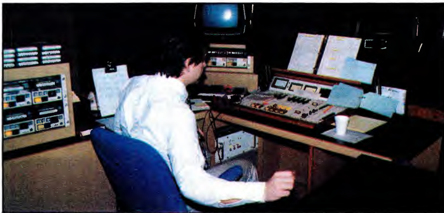
KOIT-FM's control room is equipped with a live-assist automation system and standard audio source gear.
