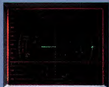
Dot placement on the +x axis indicates an error in the color frame matching of two signals.
