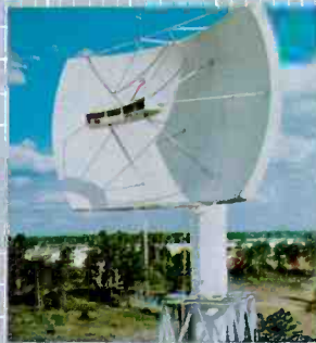
Tests conducted at Antenna Technology Corporation's range site demonstrate SIMULSAT's unique ability to simultaneously receive signals from all domestic satellites (Satcom IV at 83° west to Satcom IR at 139° west). In addition, range pattern tests show that carrier-to-interference isolation is sufficient for 2° C band spacing applications.
