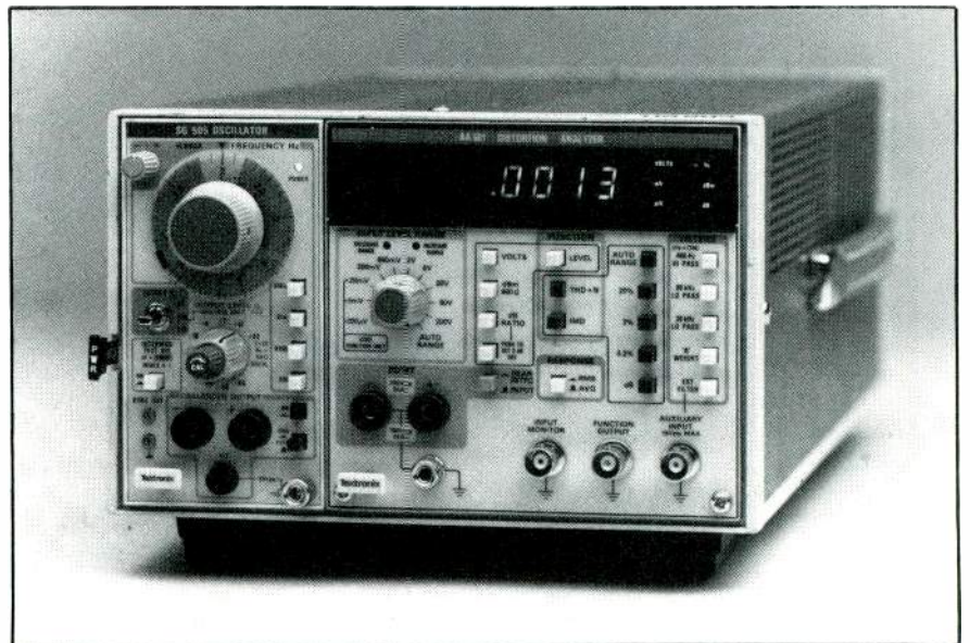
Tektronix model SG 505/AA 501 test set, an example of the new generation of audio test equipment available today.
