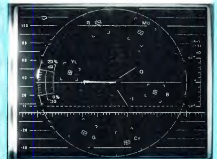
Figure 8. A timing jitter of about 6ns peak-to-peak on the selected signal's sync on the SCH display.
