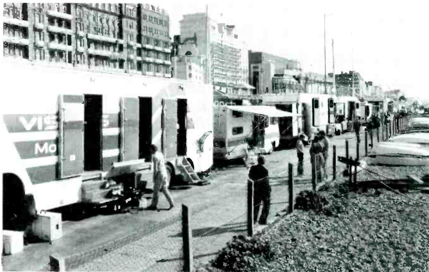
Almost a half-mile of mobile production systems lined the Brighton Promenade. Some were small units for downlinking from a single satellite, but others were complete facilities with 8 cameras and self-contained power.
