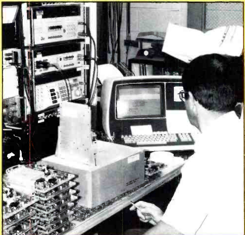
This automated printed circuit board drilling deck produces PC cards with high speed and accuracy. The data that drives the deck is generated by a CAD system.
