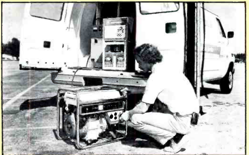
The repeater vans are each equipped with a portable gasoline-powered generator to recharge the on-board battery bank.
