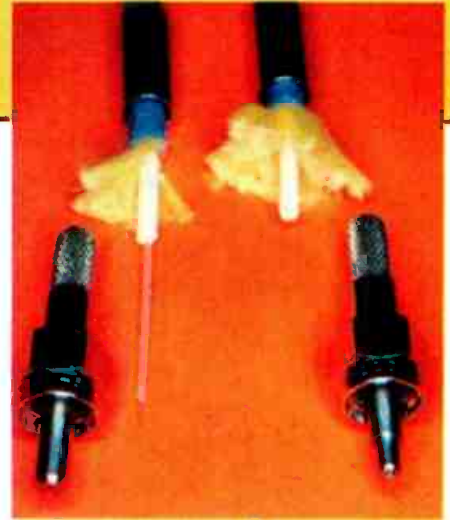
Single-fiber loose-tube cables before insertion into a connector. The buffer coating seen on the larger fiber must be removed before installation.
