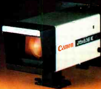
J15x8.5B1E for 2/3" cameras. 2/3" Economy—full utility for all studio situations, combining a 15X zoom ratio with an M.O.D. of under two feet, a 54° angle of view and high sensitivity throughout the range. Focal length: 8.5-128mm (17-256mm w/built-in extender) Max. Relative Aperture: 1:1.6 at all focal lengths
