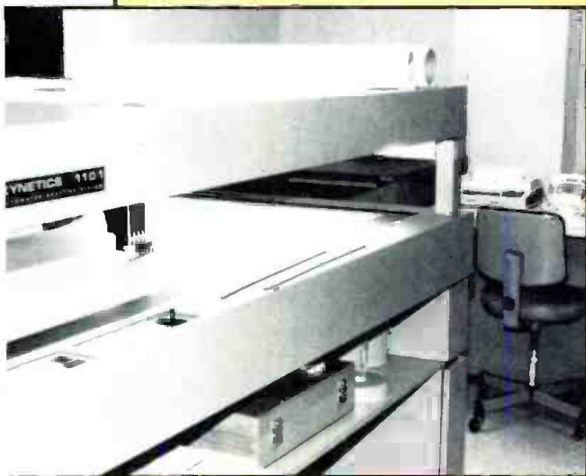
The primary output device for a CAD system is usually a graphics plotter. This unit can draw both schematic diagrams and printed circuit board layouts.
