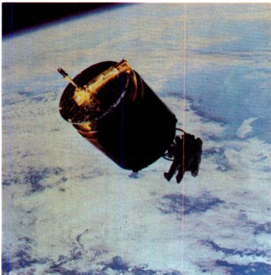
Astronaut Dale Gardner prepares to dock with the spinning Westar VI satellite using the shuttle's manned maneuvering unit. Westar VI, like the Palapa B-2 satellite, was lost in February 1984, when a rocket motor failed during transfer into geostationary orbit.
