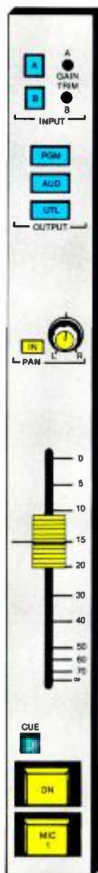
Figure 1. The layout of a typical microphone or line-level input module for use in an on-air audio console.
