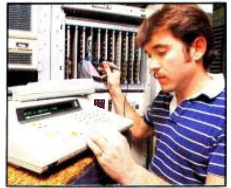
KCST-TV engineer Mike Bell troubleshoots the microcircuit that controls a character and graphics generator.
