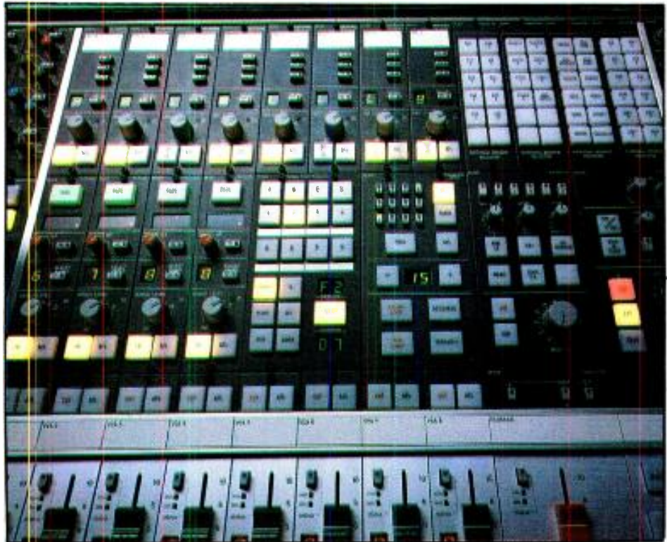
To maximize efficiency, new stereo TV audio consoles may incorporate computer-controlled switching, centralized routing assignment and specialized output configurations. (Shown is a section of the Solid State Logic SL 5000 M series audio console.)
