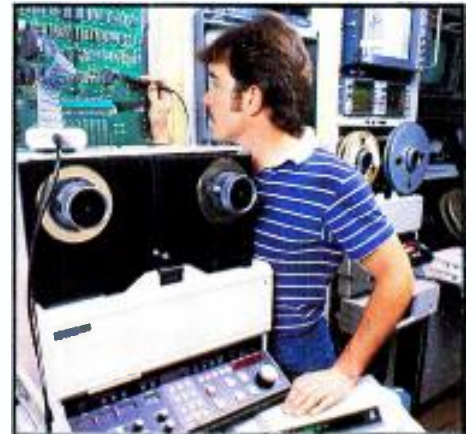
Digital malfunctions in videotape recorders can be diagnosed using the 9010A's preprogrammed functions.
