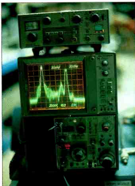
A spectrum analyzer and sideband adapter are not required, but can be a nice addition to a facility's inventory of test equipment.
