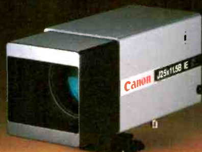
J25x11.5BIE for 2/3" cameras. Greater Reach —a 25X zoom lens designed specifically for 2/3" cameras. The power and scope of 1" systems, the economy and efficiency of your 2/3" cameras. Focal length: 11.5-288mm (23-576mm w/2X extender) Max. Relative Aperture: 1:1.6 through 220mm 1:2.1 at 288mm
