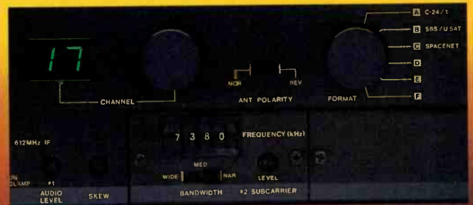
Format control enables selections of desired satellite system. Direct-reading channel selector displays transponder-assigned channel. Second selectable, subcarrier and space for optional third subcarrier or descrambler modules.
