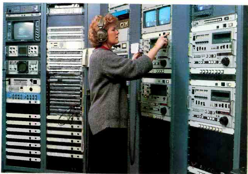
Master control switcher works together with the distribution switcher and machine control.
