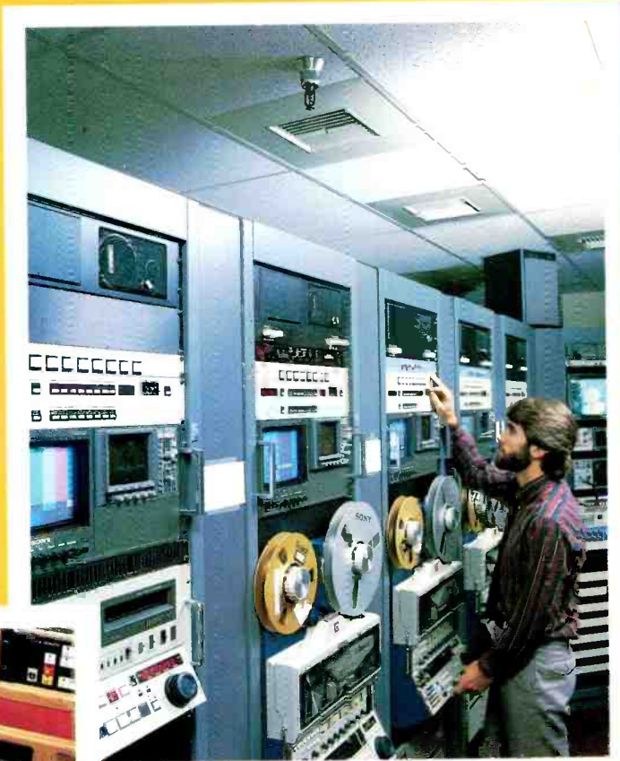
VTRs can be controlled with source selection panels and machine assignment panels.
