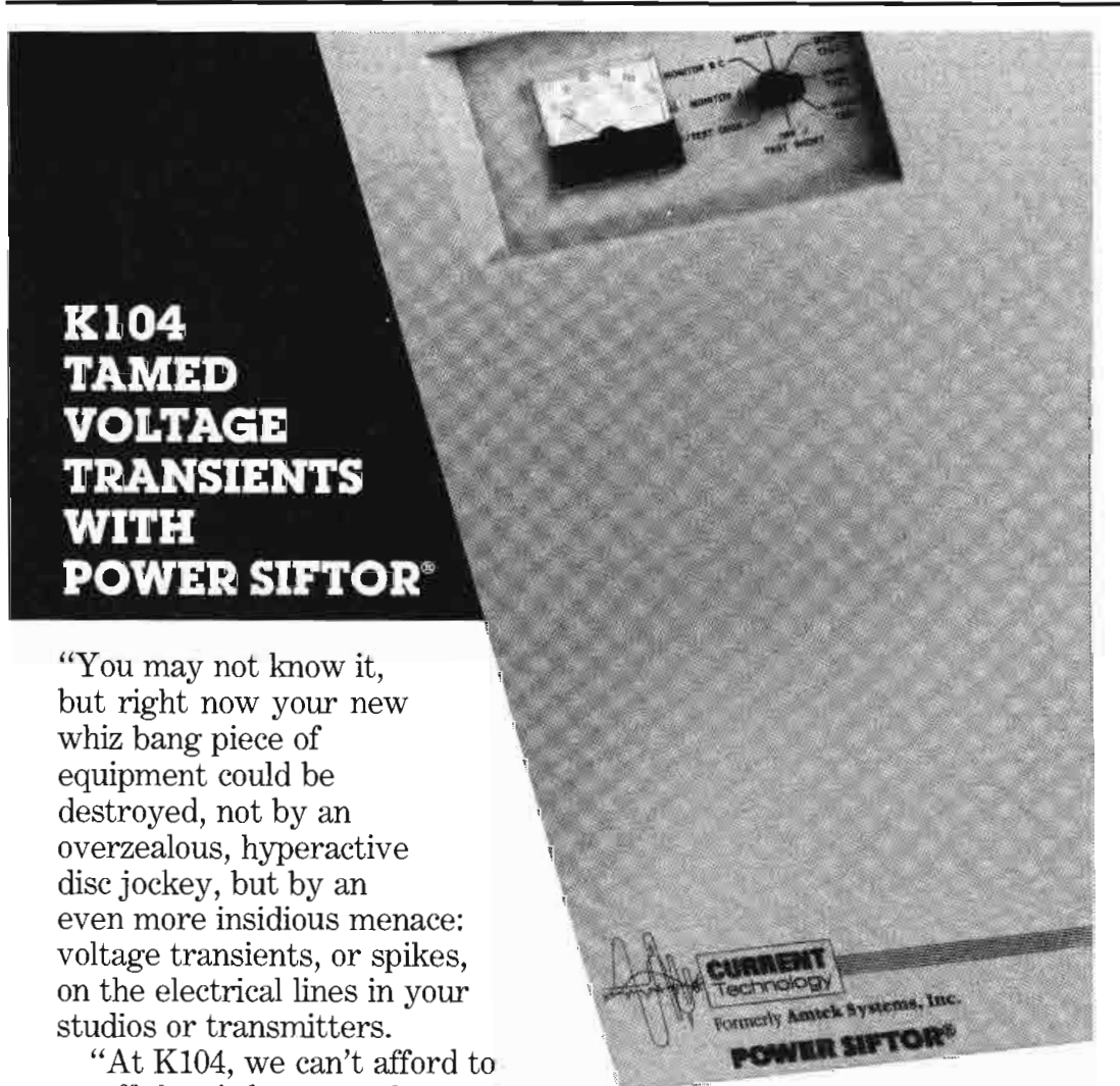
Figure 2. Spike clippers suppress only voltage spikes that exceed the clamping voltage, which is customarily set at approximately 200Vac for a nominal 120Vac power line.
