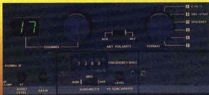
Format control enables selections of desired satellite system. Direct-reading channel selector displays transponder-assigned channel. Second selectable, subcarrier and space for optional third subcarrier or descrambler modules.
