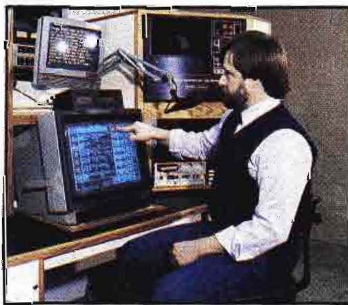
The modified color TV monitor provides control and feedback information to the operator. All control takes place by pressing the CRT screen.
