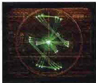
Triple Vector Overlay— SMPTE Bars on A, B and C inputs delayed by 6° and 12° to demonstrate phase error
