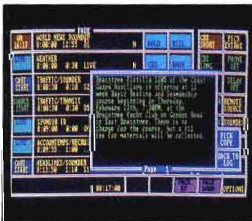
Program log and tag-copy appear in windows, which overlay the current information. The windows for a variety of information can be recalled or removed by touching the screen.
