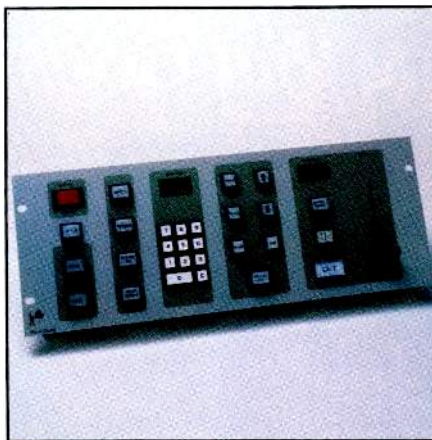
Control panels may involve defined function keys or programmable soft keys.
