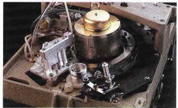
Computer-aided design techniques resulted in a pinch-rollerless transport with optimized tape path geometry, and a superior threading mechanism.
