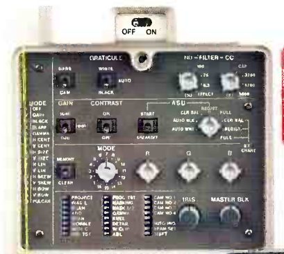
Rear panel on Hitachi's SK-970D camera. Complete controls for automatic setup and camera operation.
