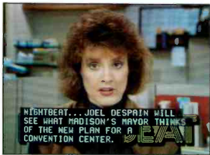
Figure 2. With a second-generation newsroom computer system, low-cost, real-time closed captioning can be achieved by routing the computer-generated teleprompter feed to the captioning encoder as well.
