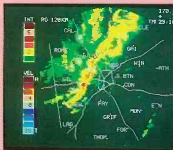
A conventional intensity display of a rainstorm over Atlanta shows different strengths with different colors. Here, green plots light rain, yellow is moderate and orange is somewhat heavy. Colors are programmed locally. Typically, six colors represent all rainfall intensities.
