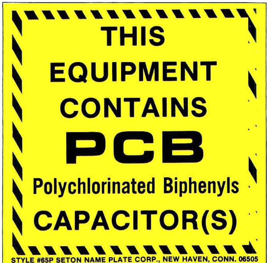
Figure 1. The large marking label (ML) is used to identify PCB transformers and PCB large capacitors.
