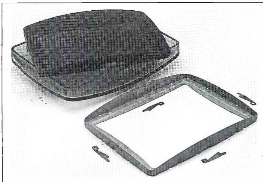
Figure 1. In conventional suspension designs, a heavy mask frame is suspended by three or four bimetallic springs engaged in studs in the middle of the faceplate walls.
