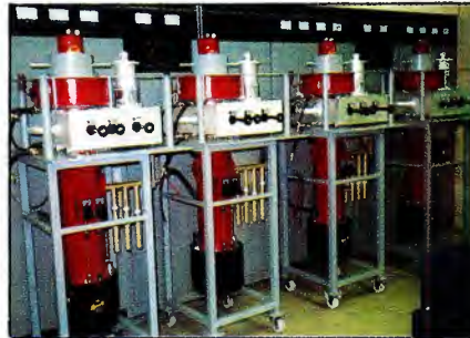
Lined up and ready to go. The three Klystrode tubes used in the WCES 120kW transmitter await installation at the GPTV station in Wrens, GA. The fourth device is a spare. (Photo courtesy of Comark.)
