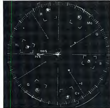
Figure 8. Vectorscope display of color bars taken during the WCES proof.
