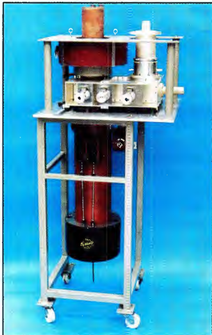
Figure 1. The 60kW Klystrode tube mounted in its support stand with the output cavity attached (a). A close-up view of the double-tuned output cavity is shown in (b). (Photos courtesy of Varian EIMAC.)
