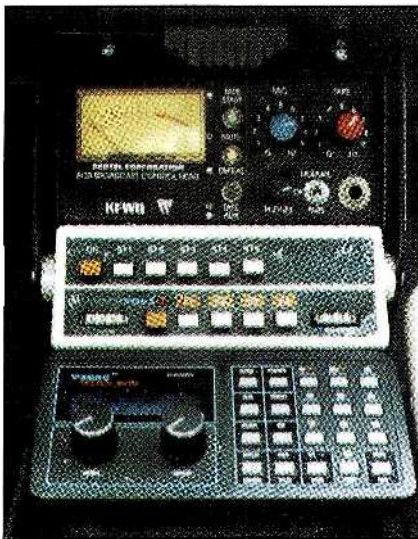
Stacking the equipment allows maximum use of space. Note the audio mixer, which permits wraparounds on both the 2-way and cellular phone.
