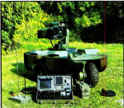
Figure 1. Tele-operated platform pays out fiber as it wanders over nearly any terrain. A fiber remote-control cable sends signals back to the operator.
