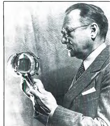
Zworykin (1940) is shown holding an early model of the iconoscope, which he developed as the all-electronic eye of the TV camera.
