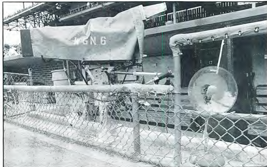
Use of surround sound at a baseball game. Two microphones in parabolic dish mounts provide detail audio. One microphone is aimed at the batter's box to capture the bat cracks of right-handed batters. The other microphone is aimed at first base. A similar arrangement is used on the third-base side.
