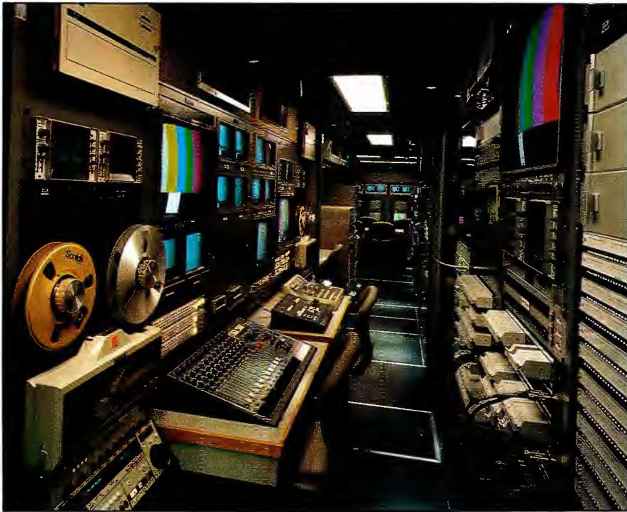
Remote production today is not unlike production at the studio. Large, complex trailers have given field producers the capability to take the tools of the trade on the road. Shown is the interior of an NBC-TV tape production van.
