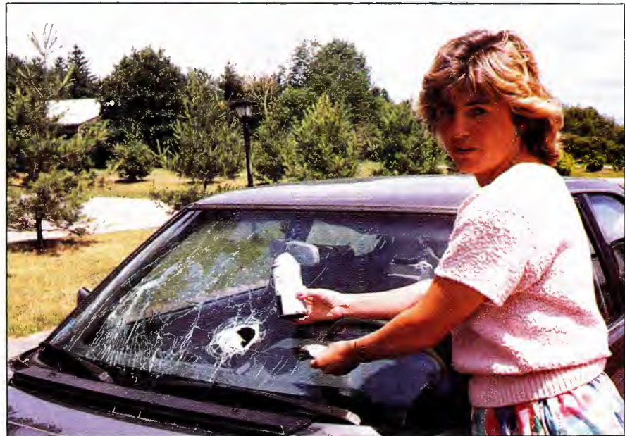
As a result of high temperatures in the car, the small aerosol can, shown here, caused severe damage to the windshield and dashboard.
