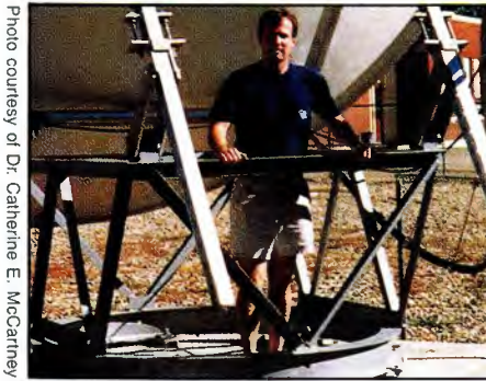
Photo courtesy of Dr. Catherine E. McCartney Lightweight dishes are especially vulnerable to warping if the dual rear support brackets are not properly adjusted. Both brackets must be moved equally to prevent misalignment of the dish focus point.
