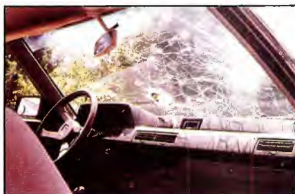
Interior dashboard damage. If the can had exploded when the car was being driven, the results could have been fatal.
