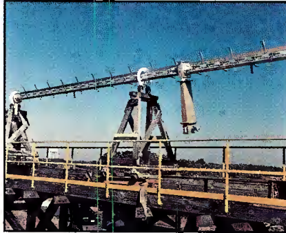
Z dipole-type variable circular polarization antenna on the test bed in Gibbsboro, NJ.
