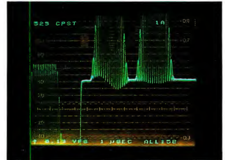
Figure 2. Dual timing pulses indicate a slight gain equality in the Y/R-Y channel, and a timing delay in the Y/B-Y channel.
