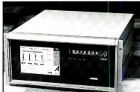
Front panel of Paragon digital audio transmission processor, showing the touchscreen control panel at left.
