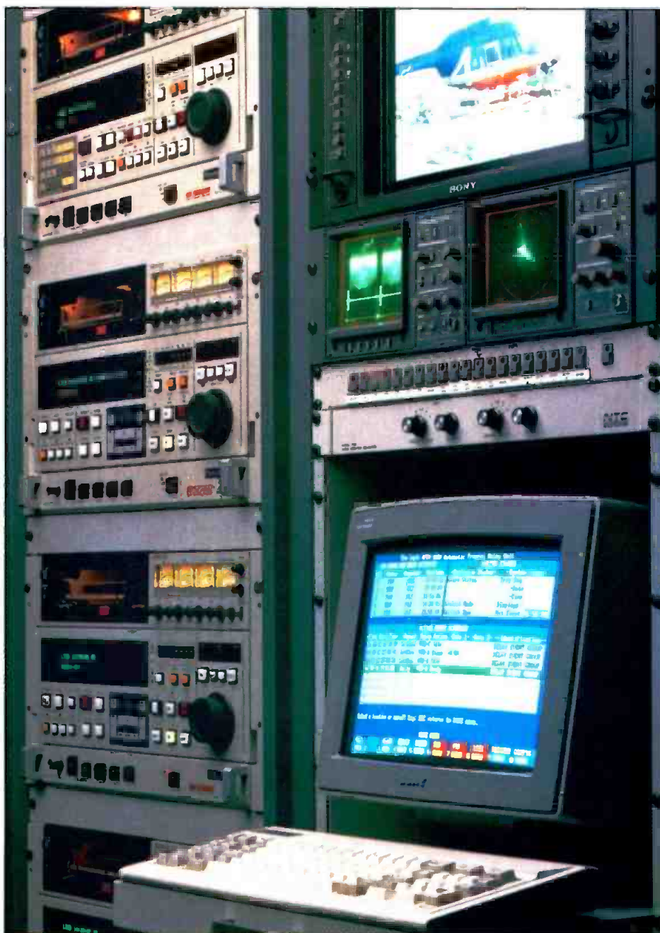
Computers can control multiple tape machines for automated recording and playback of incoming feeds. These systems also have application in network delay of broadcasts to accommodate time zones. (Photo courtesy of Time Logic.)
