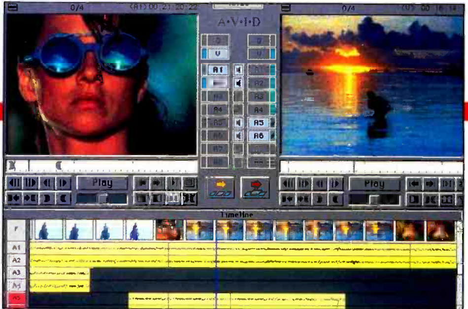
The ability of small computers to operate multiple tape machines has led to a new generation of editing systems. This user interface displays images from source and record decks, as well as giving visual representations of audio tracks. (Photo courtesy of Avid Technology.)
