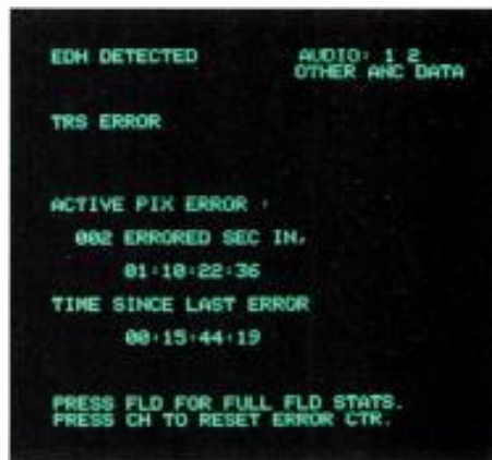
Figure 3. One possible EDH display indicates the number of program seconds that contained errors instead of a straight bit error rate number.
