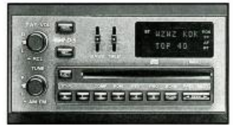
A prototype car radio equipped with an RDS display shows information about the station currently tuned in. Home receivers will incorporate larger alphanumeric displays for the RDS "radiotext" (RT) feature.
