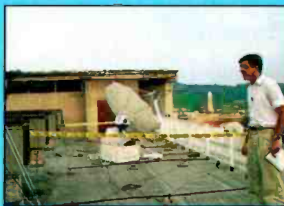
Figure 1. A flyaway satellite receiver being used in coverage of the Yugoslavian civil war. (Courtesy of Conus Communications.)
