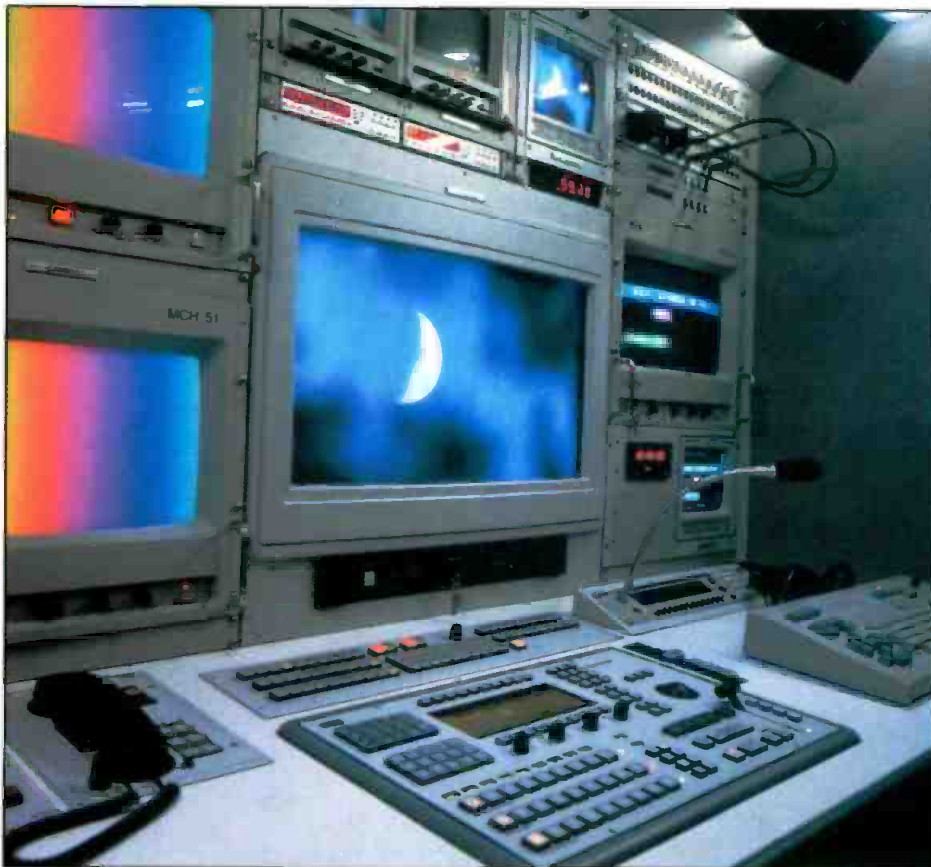
Control room inside a 2-camera HDTV OB van.
