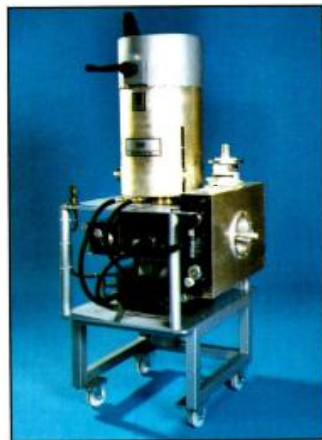
The inductive output tube (IOT) is another step in the search for higher efficiency in UHF TV power amplifiers. Although the current devices are rated at 40kW in water-cooled and air-cooled versions, a step toward 70kW can be expected in the near future.
