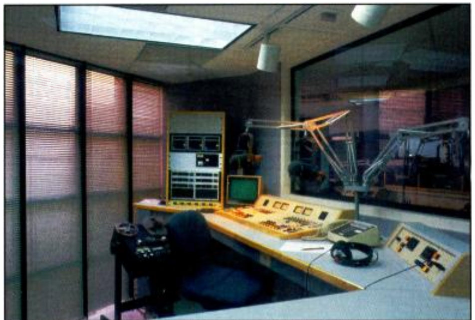
The window to the lightwell is behind and to the left of the operator's position. The mini-blinds covering the floor-to-ceiling window allow the operator to adjust the amount of light into the studio.
