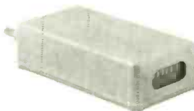
STRIKE COUNTERS TOWER/POWER/PHONE
