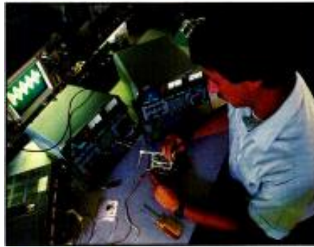
A communications service monitor is an ideal tool for troubleshooting intermod problems, as well as aligning RPU equipment. They are frequency agile for fast setup and ease of use. Many units include a spectrum analyzer.
