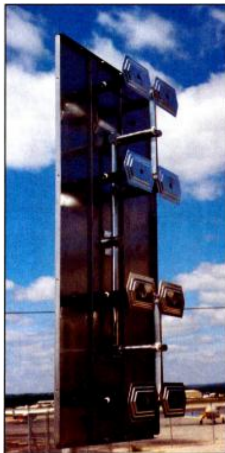
A single panel from a multichannel panel array, with radome removed.
