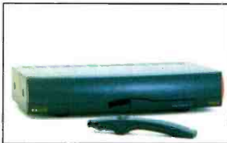
The interactive TV appliance (ITA), has 2-way capability. It contains the technology to process, encrypt and transmit/receive data that appears on the TV screen.
