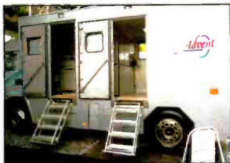
A mid-size mobile unit with separate compartments for transmission (at left door) and production.
