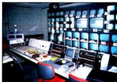
Production control room of a mobile unit, configured for ABC's Monday Night Football.
