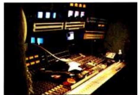
Audio control room of a mobile production unit. Window above console looks into production control room.
