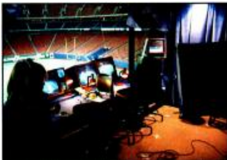
Announce booth for Monday Night Football, connected to mobile unit by multiple audio, video and intercom circuits. Booth coordinator is at left.
