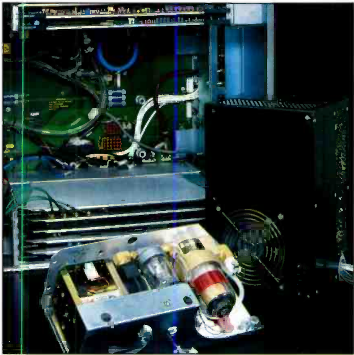
The transport assembly is modular, allowing easy access and servicing of any component.
