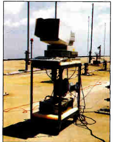
The measuring system is contained on a portable cart containing the computer, interface device and spectrum analyzer.
