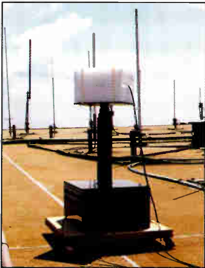
The robot was required to make measurements at two elevations. Shown here is the 3-foot level.
