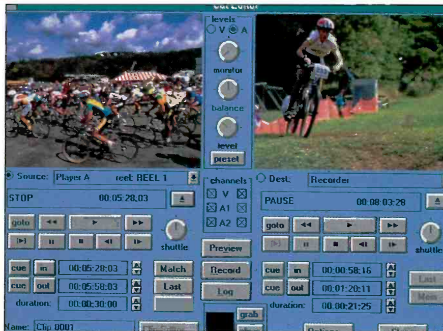
Screen shot of a PC-based editing system showing machine controls, video and edit points. (Photo courtesy of Matrox.)
