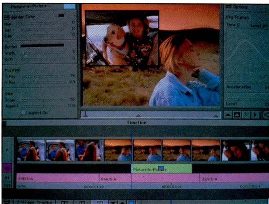
The effects mode available on a Mac-based non-linear editor. Pictures along time lines indicate shots used and relative lengths. Pull-down menus allow quick setup of parameters and options. (Photo courtesy of AVID.)
