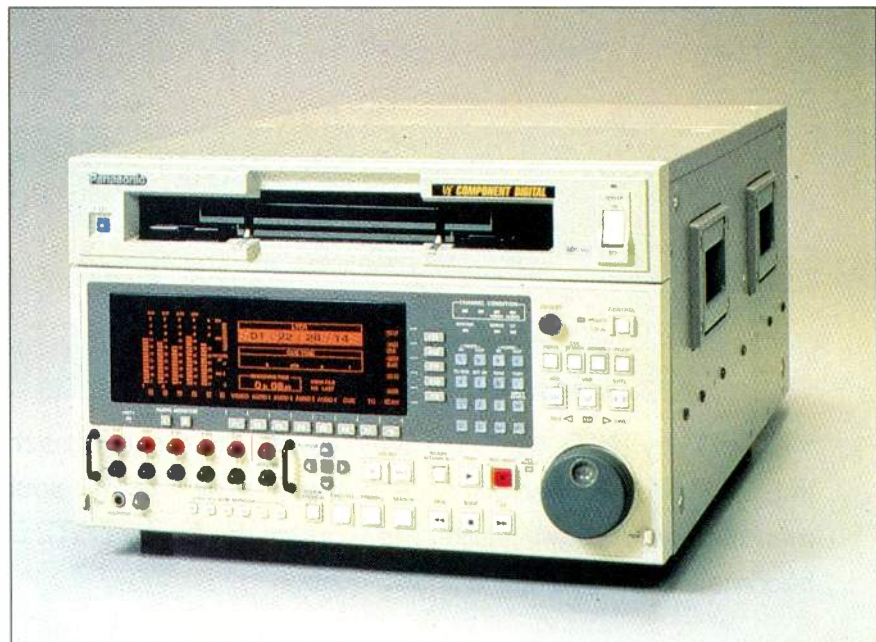
The Panasonic AJ-D580, a D-5 component digital VTR.
