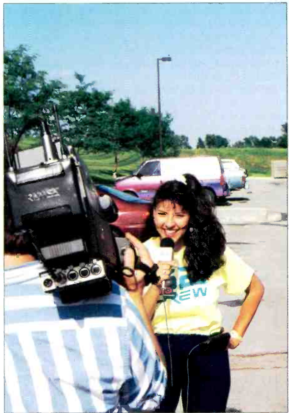
Camcorder-mounting of WX-RP700 receiver, along with hand-held microphone feeding WX-RP410 belt-pack transmitter, shown during KSMO-TV's evaluations.
