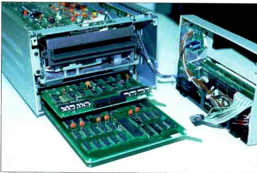
Dip switches on the CPU board provide many options for control of the unit. The switches are accessible while the unit is rack mounted. (Photo by Jon DeHart.)
